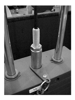
Figure 8. Screw the cable into the weight stack.
